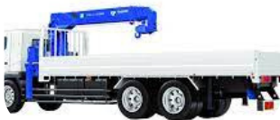
Boom Truck (10–12 Ton)
